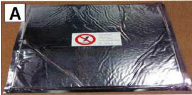
FIGURE 2 This is Phase 18C PCM Pack out of the Crate. It's the Top because of this warning label to be careful when manipulating. The actual identification label shows that it can be used in both places
