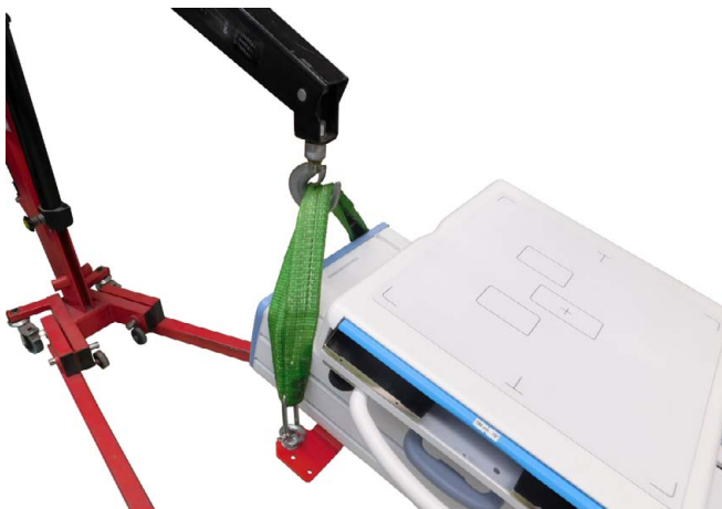
Illustration 3-5 Wall Stand Lifting
