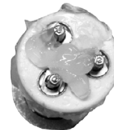
HV Cable Terminal with Silicone Paste
