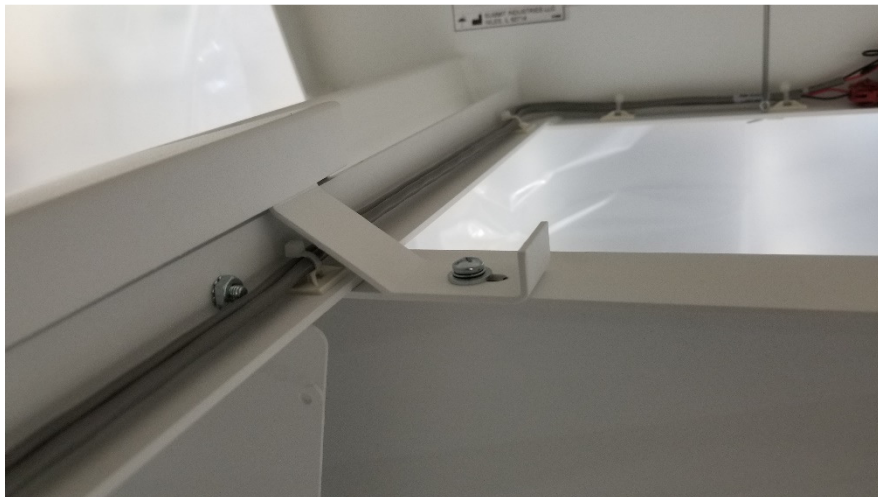
Figure 36: Fixed Front Cover Brackets
