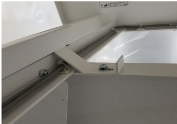
Figure 31: Fixed Front Cover Brackets
