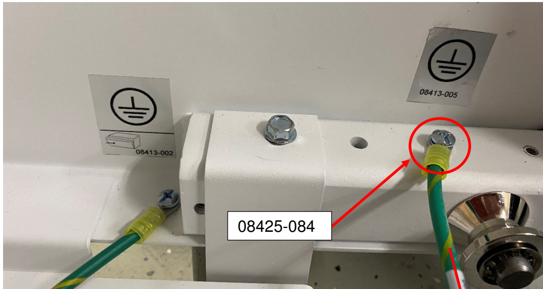
Figure 23: Earth connection in table
