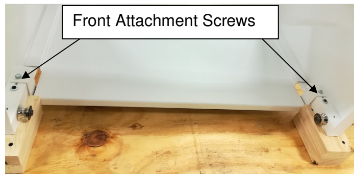
Figure 3: Table Front Attachment to Skid
