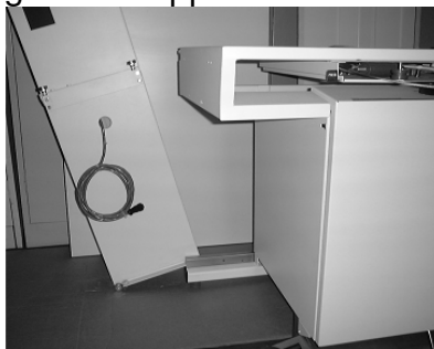
Figure 5: Mounting Tubestand to Lower Rail
