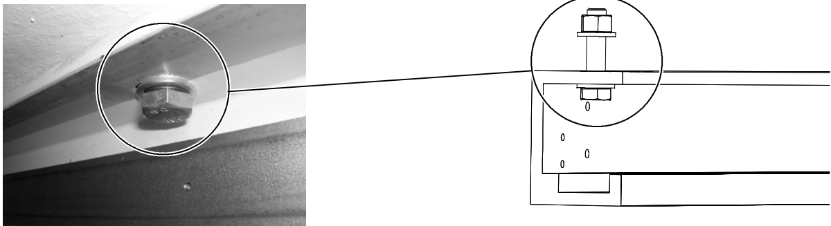
Illustration 2-2 Fix Longitudinal Rails to Ceiling
