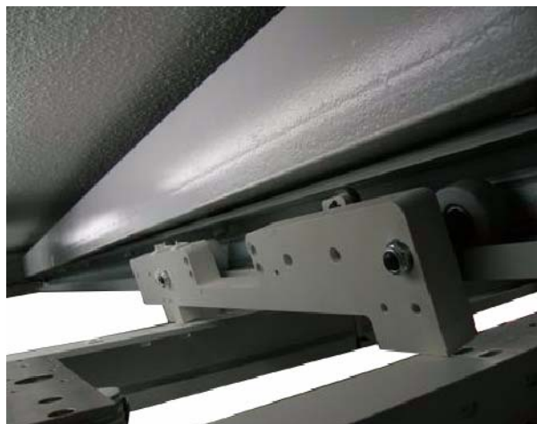
Illustration 2-40 Place the Fixation Bearing in the correct position
