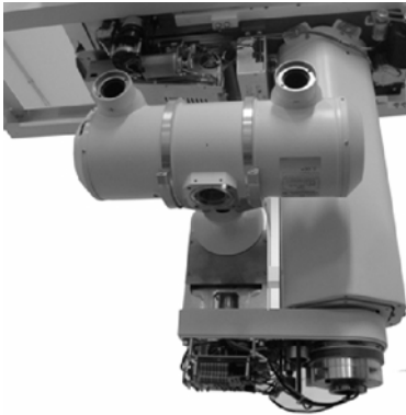
Illustration 2-76 Center the Tube and fix all Holders
