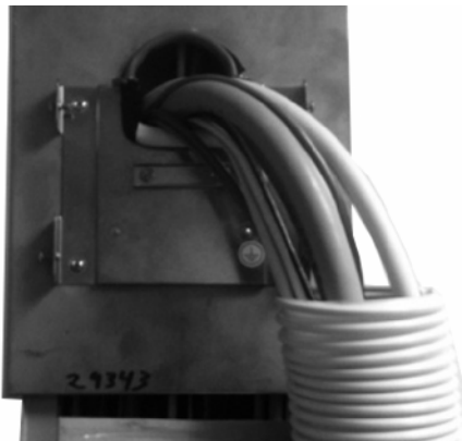
Illustration 2-104 Hose Wall Support Installation
