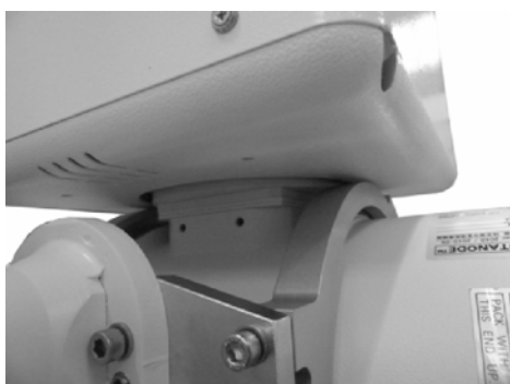
Illustration 2-83 Spacers and Fixation Points
