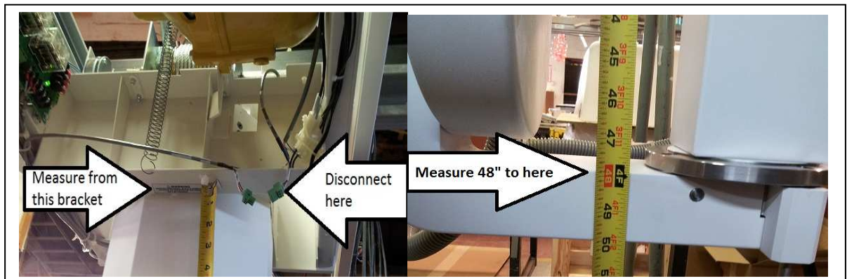
Figure 3-8 Procedure to Calibrate Vertical SID Pot
