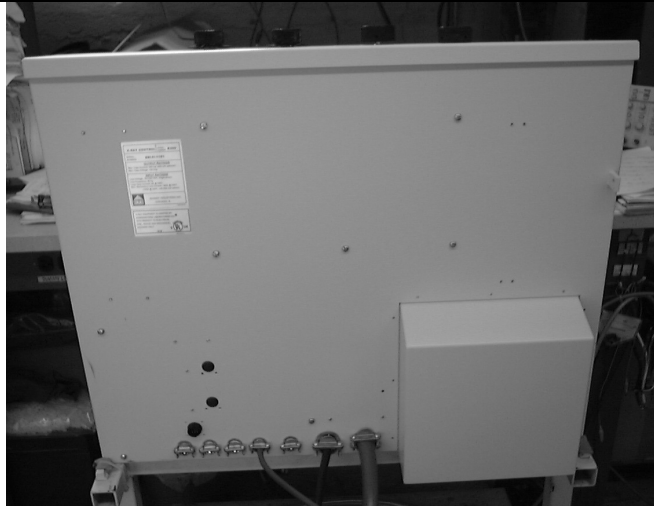
Cable Entry Points at rear of Control
