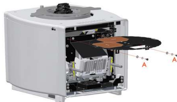
Fig. Filter substitution
