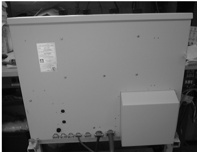
Figure 15: Rear of Control Showing Cable Entry Points
