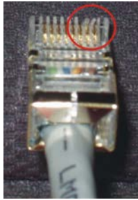
Figure 2-3: A damage example of Console cable connector
