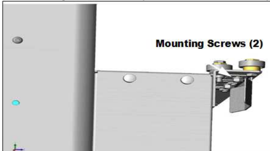
Figure 21: Mounting of interlock ramp bracket to tubestand adapter box
