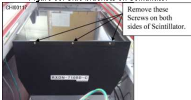
Figure 38: Side brackets on Scintillator
